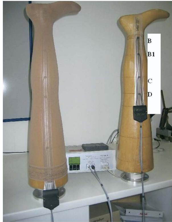
**Fig 1.** Measurement of interface pressure by medical stocking tester (MST). The measuring points are B, ankle; B1, gaiter area; C, largest calf circumference; and D, below knee.
